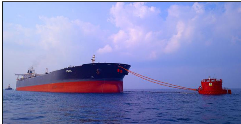
Figura 2-16 Transferencia de aceite Single Buoy Mooring (SBM). ( www.shipswiki.com )
