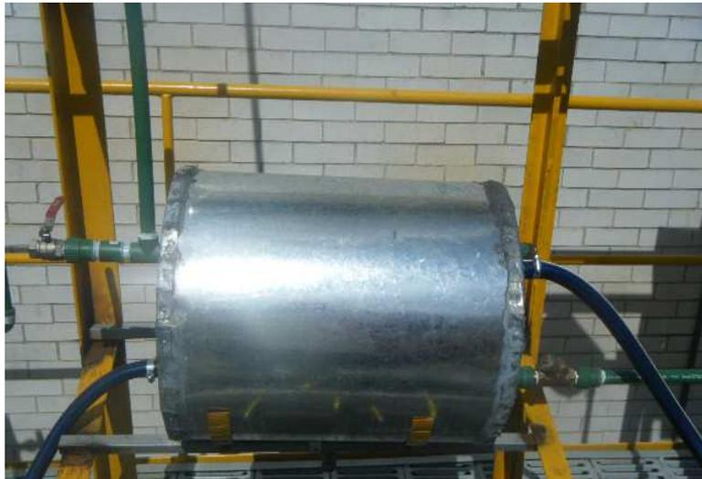
Figura 3.2 Termotanque experimental
